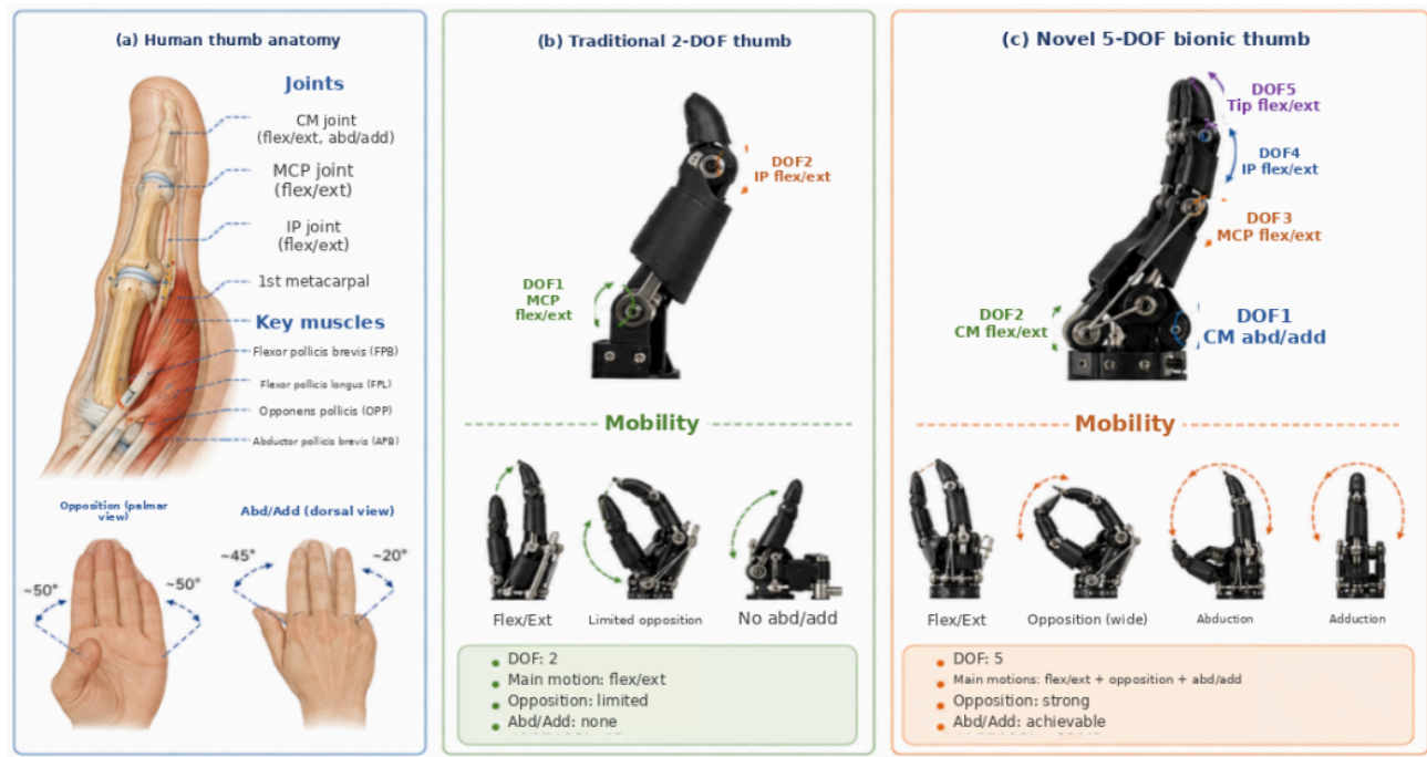
Figure 3. Comparison of biomimetic thumb opposition mechanisms
