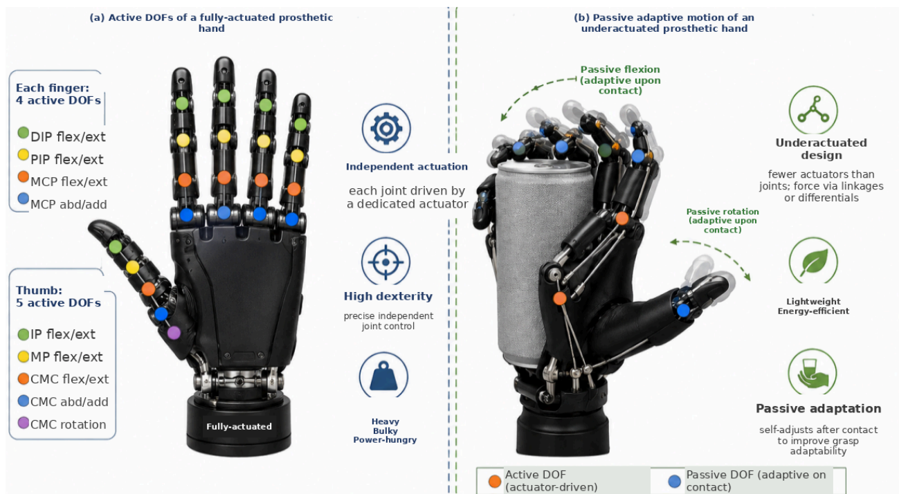
Figure 1. Schematic comparison of active and passive degrees of freedom
