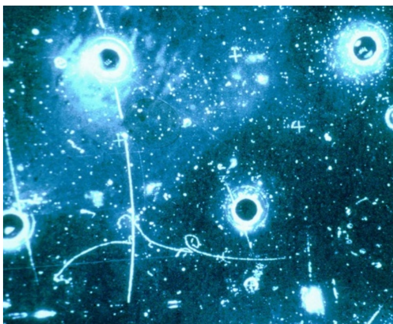
Figure 1. Neutrino tracks in the CERN Gargamelle bubble chamber [7]
