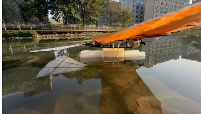
Figure 17. Illustration of flapping-wing robot floating on the water surface
