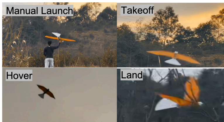
Figure 16. Illustration of aerial flight of flapping-wing robots
