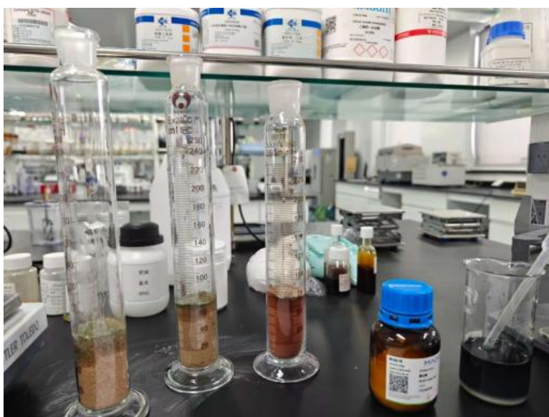
Figure 8. Diffusion experiment of lanthanum oxide in different soil media
