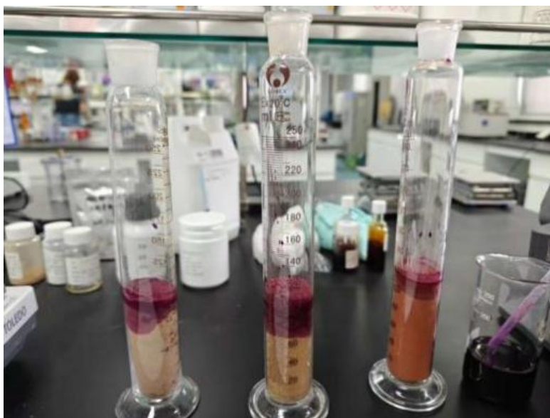
Figure 7. Diffusion experiment of potassium permanganate in different soil media
