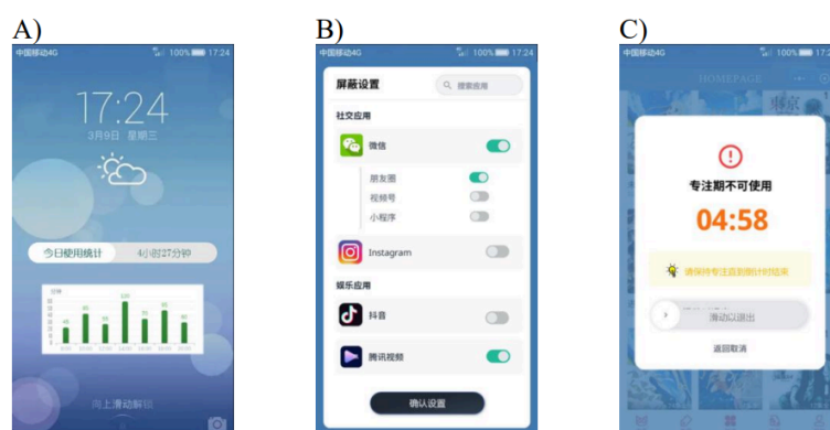
Figure 9. Prototype design of the smartphone application for regulating screen use. (A) Lock-screen interface displaying daily screen time and usage statistics, accompanied by reminders to encourage reduced exposure. (B) Selective blocking function allowing users to choose specific applications or sub-pages for restriction. (C) Blocking notification window that prevents access to selected apps or pages during focus periods, while preserving essential communication functions
