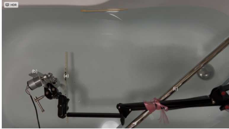
Figure 7. Set up of the experiment showing equipment involved in water wave generation itself. (a) a self-assembled Lego structure to create a planar wave, with a linear impact. (b) a miniature reciprocating motor to operate a fixed frequency. (c) an iron rod for the support of the how structure
