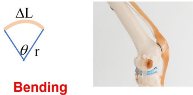
Figure 6. Working principle of the strain sensor
