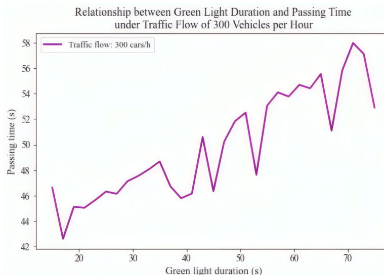
Figure 1. The relation between green light duration and passing time at 300 cars/h traffic flow
