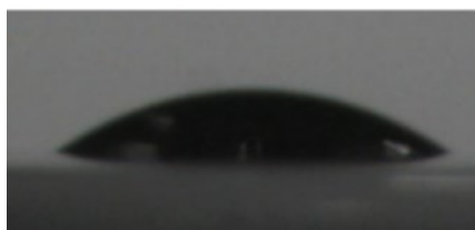
Figure 5. Contact angle photographs of the electrode surfaces of GCE/PEDOT-citrate/AuNPs/Y-shaped peptide [20].
